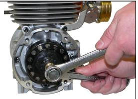
15/ Place a 17mm spanner on the Retention Nut & a 19mm spanner on the Starter Bolt. Tighten Starter Bolt against the Retention Nut until tight. Important - make sure the Retention Nut does not move in or out while tightening the starter bolt and Retention Nut together. This will effect the end float of the sprocket. End Float should be around 0.5mm
