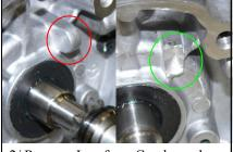
2/ Remove Lug from Crankcase by machining or with a grinder
