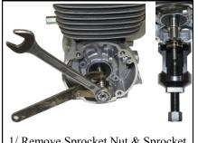
1/ Remove Sprocket Nut & Sprocket
