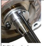
7/ Tighten the three screws evenly using a T20 Torque Screw Driver
