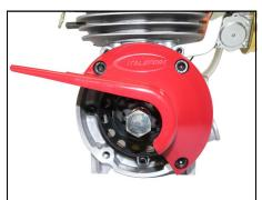
16/ Fit Clutch Guard with the three 8mm Bolts provided
