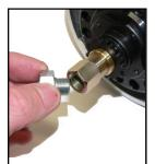
14/ Screw in Drive Bolt until it bottoms out.
