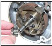
9/ Place Bearing & Bearing Sleeve on the crankshaft with the collar facing outwards.
