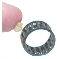
8/ Lightly grease bearing with High Temperature Bearing Grease.
